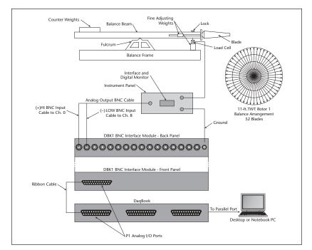
The balance flexure beam assembly is rigged to statically measure the moment weight of the compressor blades, one at a time. The output of the digital monitor connects to a DBK1 interface, which, in turn, connects to the IOtech DaqBook to collect the data. The graphics file for all the rows of blades are posted on a Microsoft Word document and printed out graphically for sorting and positioning the blades.
